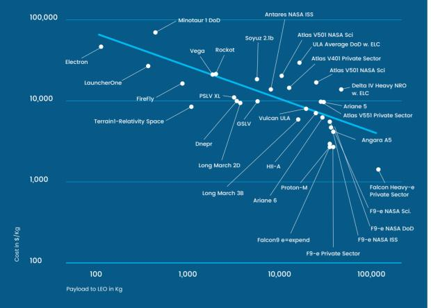
LAUNCHER CLASSIFICATION BY SIZE Source: HIE HEAVY-LIF1 MEDIUM-LIFT LIGHT-LIFT MICRO-LIF1 PAYLOAD TO LEO PAYLOAD TO LEO PAYLOAD TO LEO PAYLOAD TO LEO > 10,000 kg 4000 - 10,000 kg 500 - 4,000 kg <= 500 kg ESTIMATED **ESTIMATED ESTIMATED ESTIMATED** LAUNCH PRIZE LAUNCH PRIZE LAUNCH PRIZE LAUNCH PRIZE \$45 - 400 M \$30 - 400 M \$5 - 50 M \$1 - 10 M
